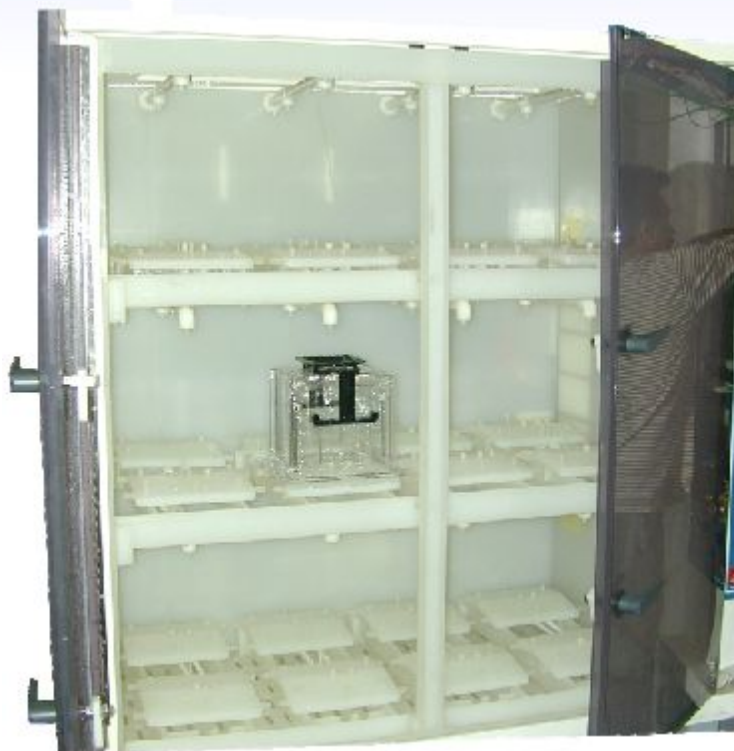
Simple ergonomic loading of wafer boxes. Interchangeable fixturing for multiple configurations of boxes, cassettes or SMIF Pods
