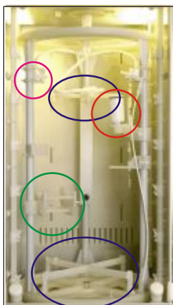
Universal boat fixture Universal thermocouple fixture Quartz baffle holder Injector
