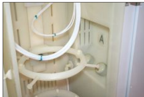
Tube retainer adds extra security. Multiple injector ports provide efficient cleaning for gas ports.
